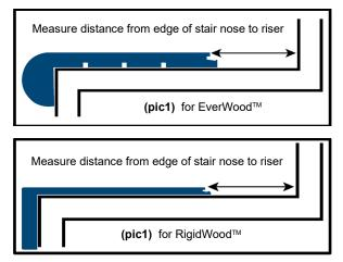
6. Connect the cut flooring to the stair nosing and dry-fit **before gluing it into place**\*\*.
