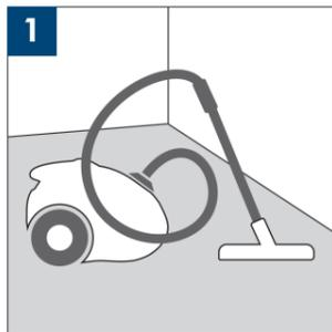
**1** Before installation begins, make sure the subfloor surface is clean, dry\*, smooth and flat. The underlay is not intended to level major subfloor imperfections.
