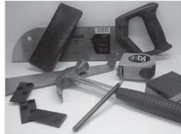
When sawing pieces off the tiles, use a fine-toothed hand saw, jigsaw, chop-saw, guillotine or utility knife.
